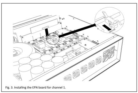
Attach the grounding wire to its connector attached to the underside of the lid and screw the lid back on. When removing the EFN module(s), move jumper J1 back to its original position, otherwise the signal path to the power amplifier is interrupted and the amplifier will not work!
