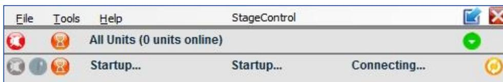
Important note: Startup will only appear for 15 seconds after powering on
