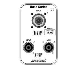
Connectorpanel of the XL-bin(S) with one 8-pole- and two 4-pole Speakon connector.
